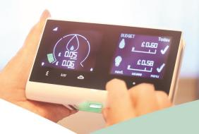
Typically used by gas and electricity companies, smart water meters are becoming more mainstream. They work by measuring your consumption and relaying the information to the utility at shorter intervals. Regular meters are read at the beginning and end of a particular period and billed accordingly.
